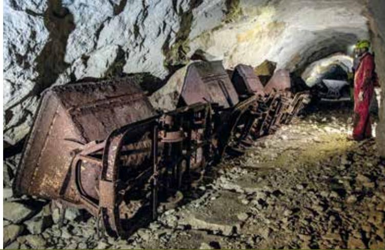
110. Left: Torretta mine, Roccamorice. Trolleys for transporting extracted rocks to the exterior.
